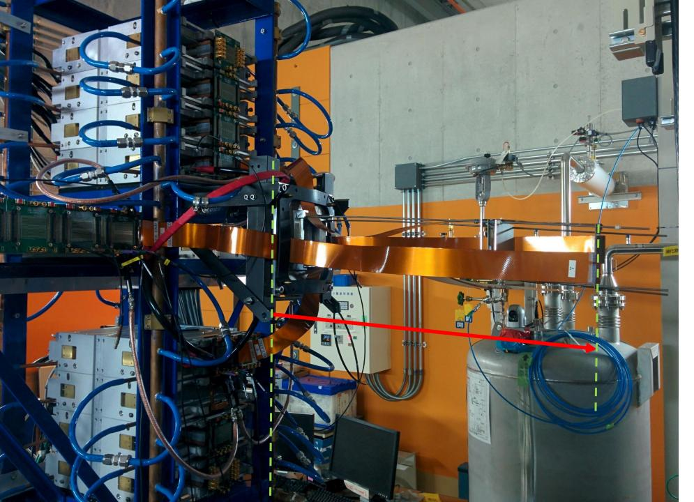
Furthest a DSSSD can go from the base of the snout ~ 54cm (~ 60cm from main Cu pipe).
