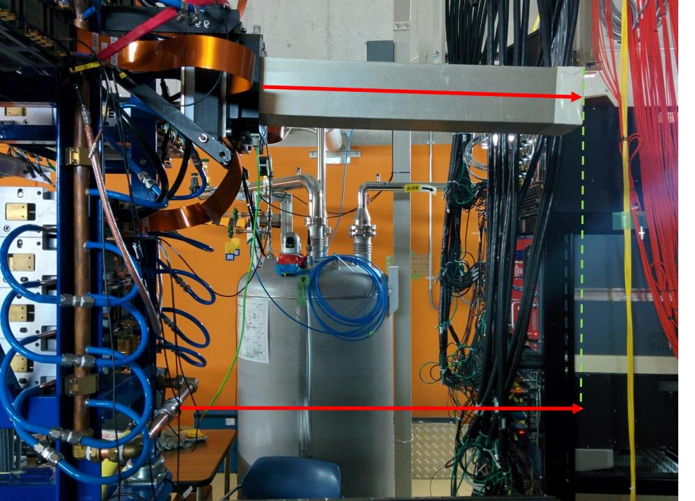
Cu cooling pipe to end of snout ~75cm
