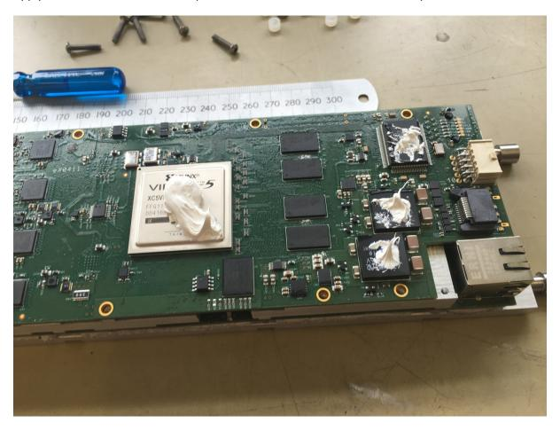
Replace the plate carefully on the pcb and install the screws and spacers loosely. Install the steel spacers in the correct positions.
