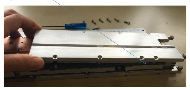
This is how it can look when the lid is off. The thermal pads may stay on the pcb. Either is fine.
