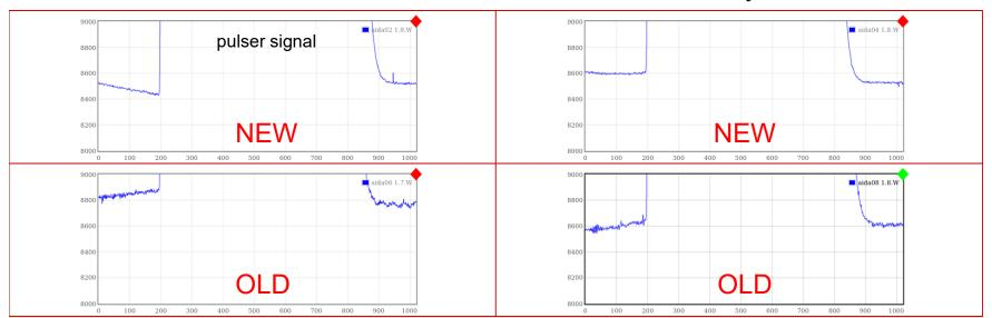
Per strip preamplifier outputs – no cabling or DSSSD – y-axis = 122mV, x-axis = 20µs
